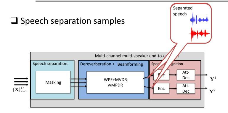
□ The mask-based neural beamformer and speech recognition are jointly optimized via ASR objective.
