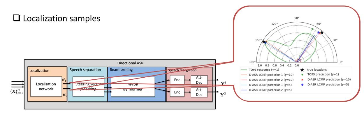
□ The localization network, mask-based neural beamformer and speech recognition are jointly optimized via ASR objective
