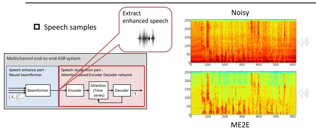
Entire network are consistently optimized with ASR-level objective including speech enhancement part
