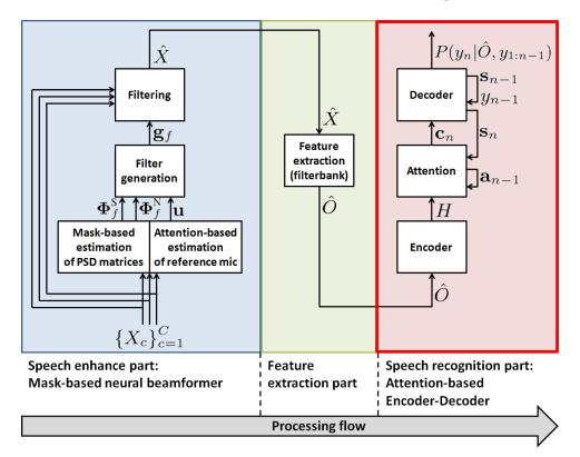
Based on a lot of **signal processing oriented** components!
